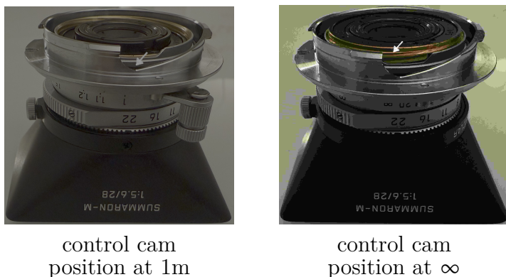
Figure 9: Notch and a control cam on a lens
